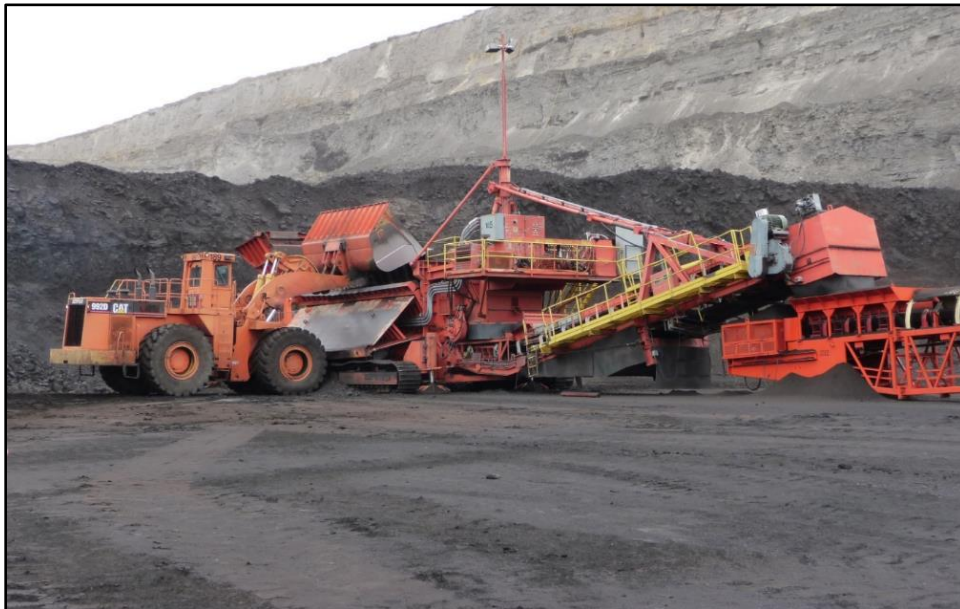
Photo 16-2: Example of a Loader Loading a Track Mounted Feeder Breaker
