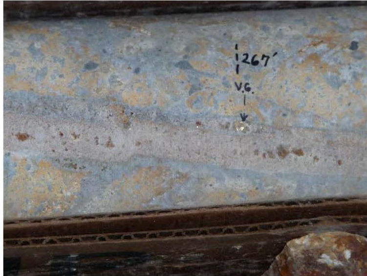
Figure 7-14 Visible Gold in Late-Stage Quartz Veinlet in Drill Hole 08 OKC-193
