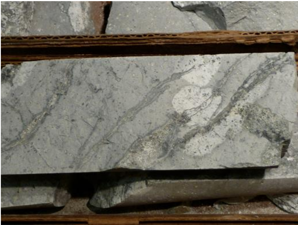
Figure 7-7 Typical bleached, hydrothermally altered Tertiary biotite rhyolite (Tpr)
