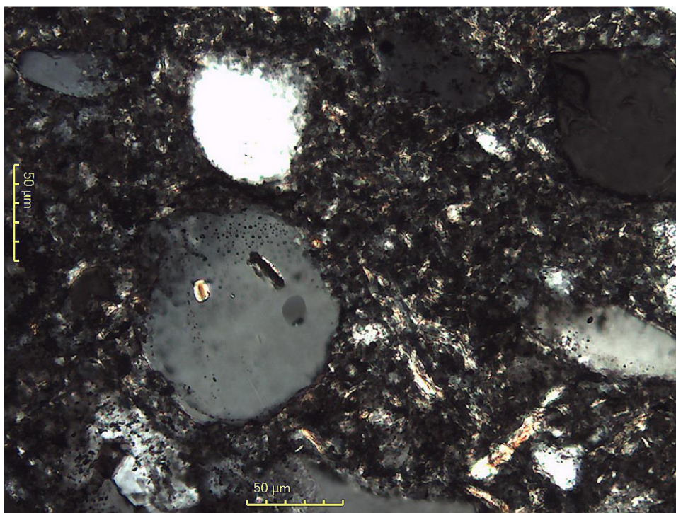
Figure 13-21 Aspen Top Drum 10 - Quartz/feldspar clasts cemented by secondary silica – 200X PL
