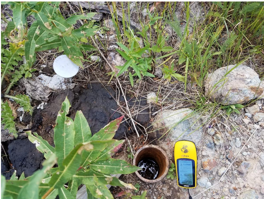
Figure 12-2 Closely Spaced, Variably Marked Drill Hole Collars
