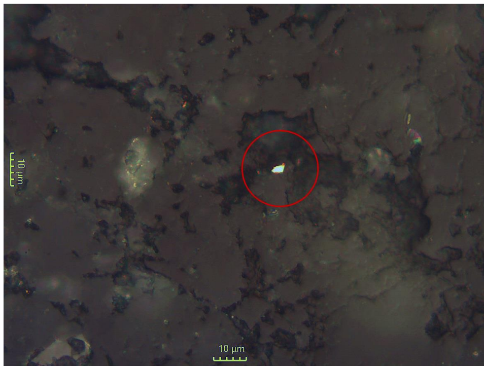
Figure 13-23 Aspen Sill Drum 13 - Bright 4 \mu m grain of Au in porphyry fragment – 500X RL
