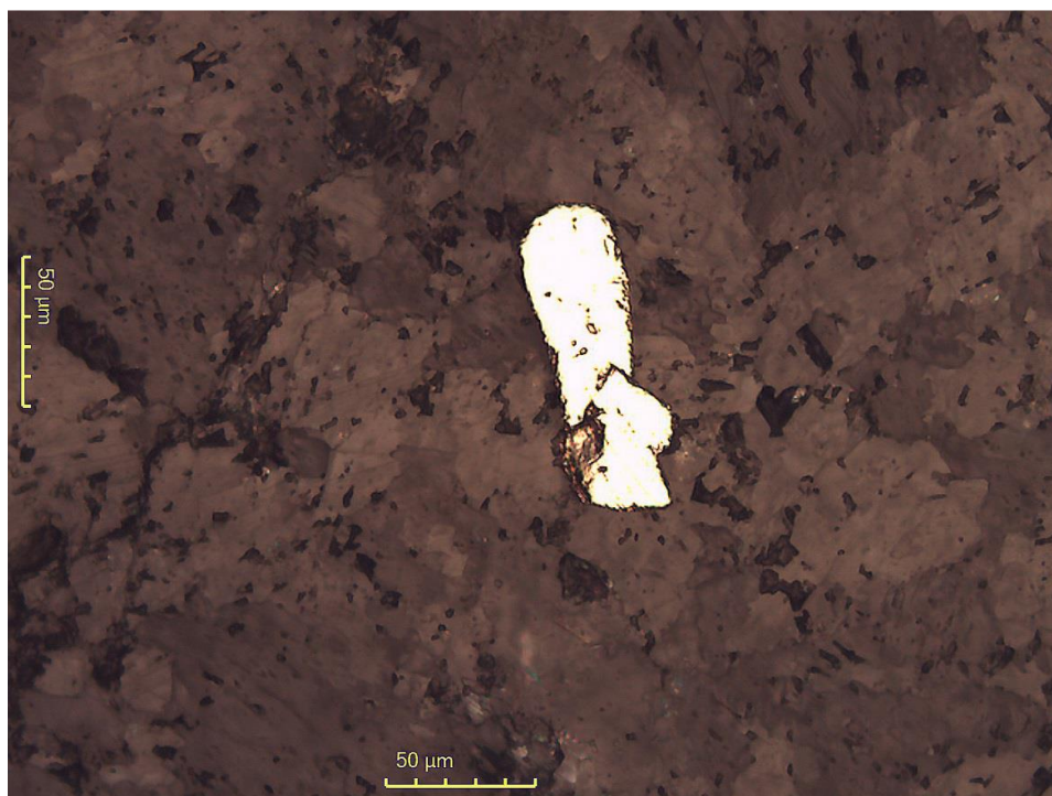
Figure 13-7 Aspen Bottom Drum 2 - Odd shaped grain of pyrite in coarse calcite – 200X RL
