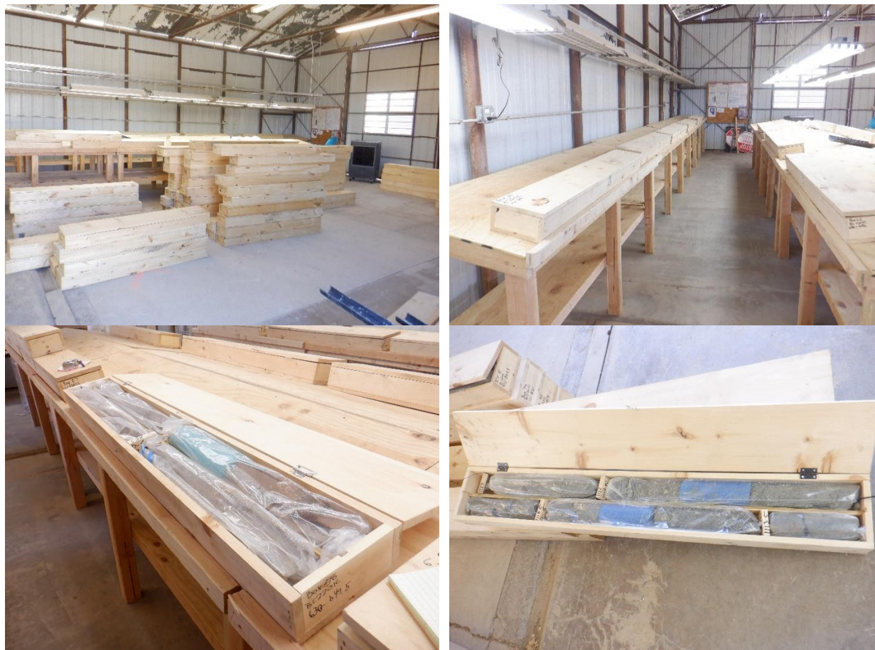
Photo 11-3: Wooden Core Boxes in the Locked Storage facility (upper photos), Core Sample from BC2201C (lower photos)
