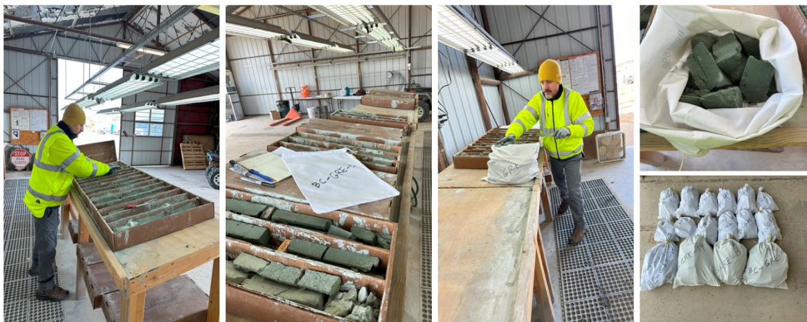
Photo 12-7: Visual Sample Inspection, Sampling, and Packing by GRE's QP in the Storage Facility
