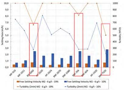
Flocculants SNF-7520 (flocculant currently employed at MVC) and SNF-704 (flocculant of interest to MVC) were used for further settling tests. Settling flux testing was performed to determine optimum dilution. These results are presented in Figure 13-8.
