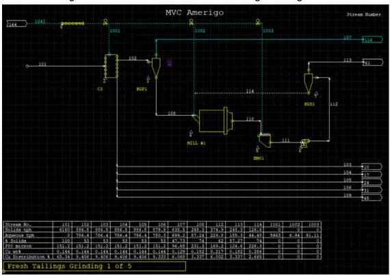
Figure 17-2: MVC MetSim Model – Fresh Tailings Grinding Line 1
