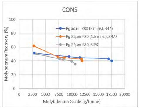
Similar to the rougher tests, the cleaner performance of the undersize feed sample was very poor for both samples. Copper and molybdenum recovery from the TEN -106  $\mu$ m samples were 9.1 and 4.0%, respectively, at a final concentrate grade of only 8.7% copper and 1881 ppm molybdenum (Figure 13-25).
