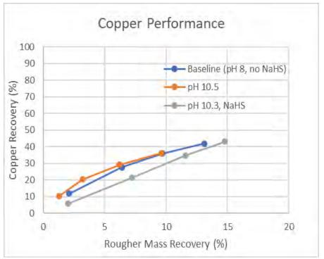
Figure 13-17: Effect of pH and NaHS on TEN Fines – Copper
