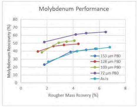
The primary grind size over the range of 72 and 217  $\mu$ m P80 was investigated for both samples. Tests were conducted at a pulp pH of 8, modified using lime. The reagents used included Aero 3477, which is a strong dithiophosphate, and MolyFlo, a hydrocarbon-based molybdenum collector. As indicated by the mineralogical analysis on the feed material, liberation for copper in the sample is poor, and further
