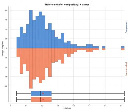
Figure 14-8: Comparison of the Uncomposited and Composited Values for the K-ratio
