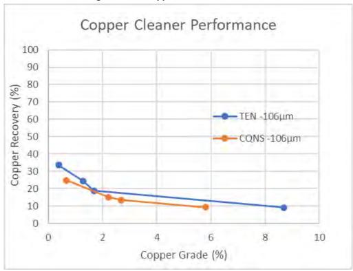
For the CQNS -106  $\mu$ m sample, results were also poor, with copper and molybdenum recoveries of 9% and 11%, respectively, at a final concentrate grade of 5.8% copper and 9579 ppm molybdenum (Figure 13-26).
