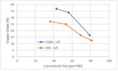
Sulfur grades were generally inversely proportional to copper grades, indicating improved performance as a result of pyrite rejection. The regrind improved liberation of copper sulfides from pyrite, leading to improved rejection of liberated pyrite.
