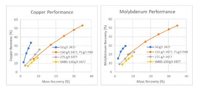
Figure 13-32: CQNS Fines - Copper and Molybdenum Fines Rougher Flotation
