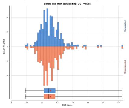
Figure 14-5: Comparison of the Uncomposited and Composited Values for CuT
