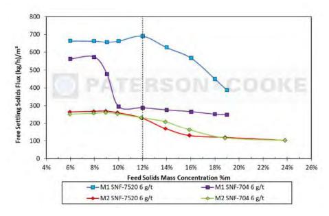
Figure 13-8: Feed Dilution Tests for M1 and M2 using SNF-7520 and SNF-704
