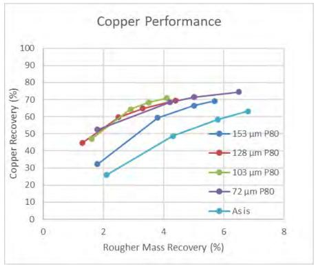
Figure 13-15: Effect of Primary Grind Size on CQNS Performance – Copper
