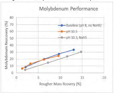
Figure 13-18: Effect of pH and NaHS on TEN Fines - Molybdenum
