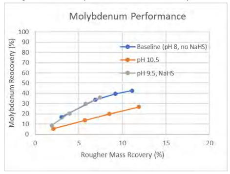
Figure 13-20: Effect of pH and NaHS on CQNS Fines – Molybdenum
